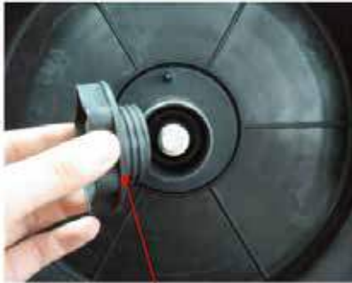
(1) Remove the spool retaining nut.
