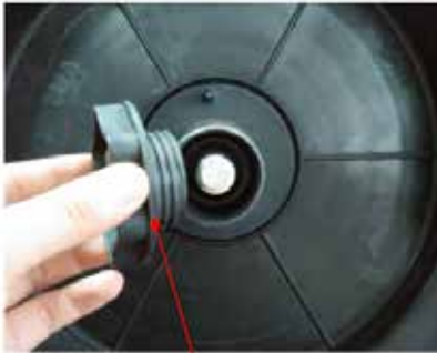
(1) Remove the spool retaining nut.
